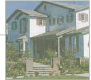
^ A semi-private entry porch and permeable fencing have been used here effectively to address the front street positively.
